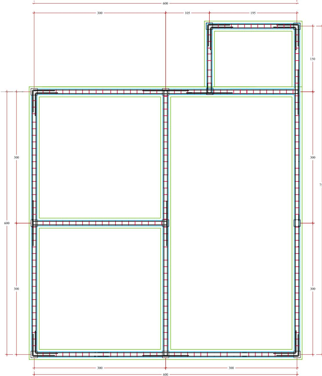
Denah Pembesian Sloof/Lay Out of Sloof Bar
