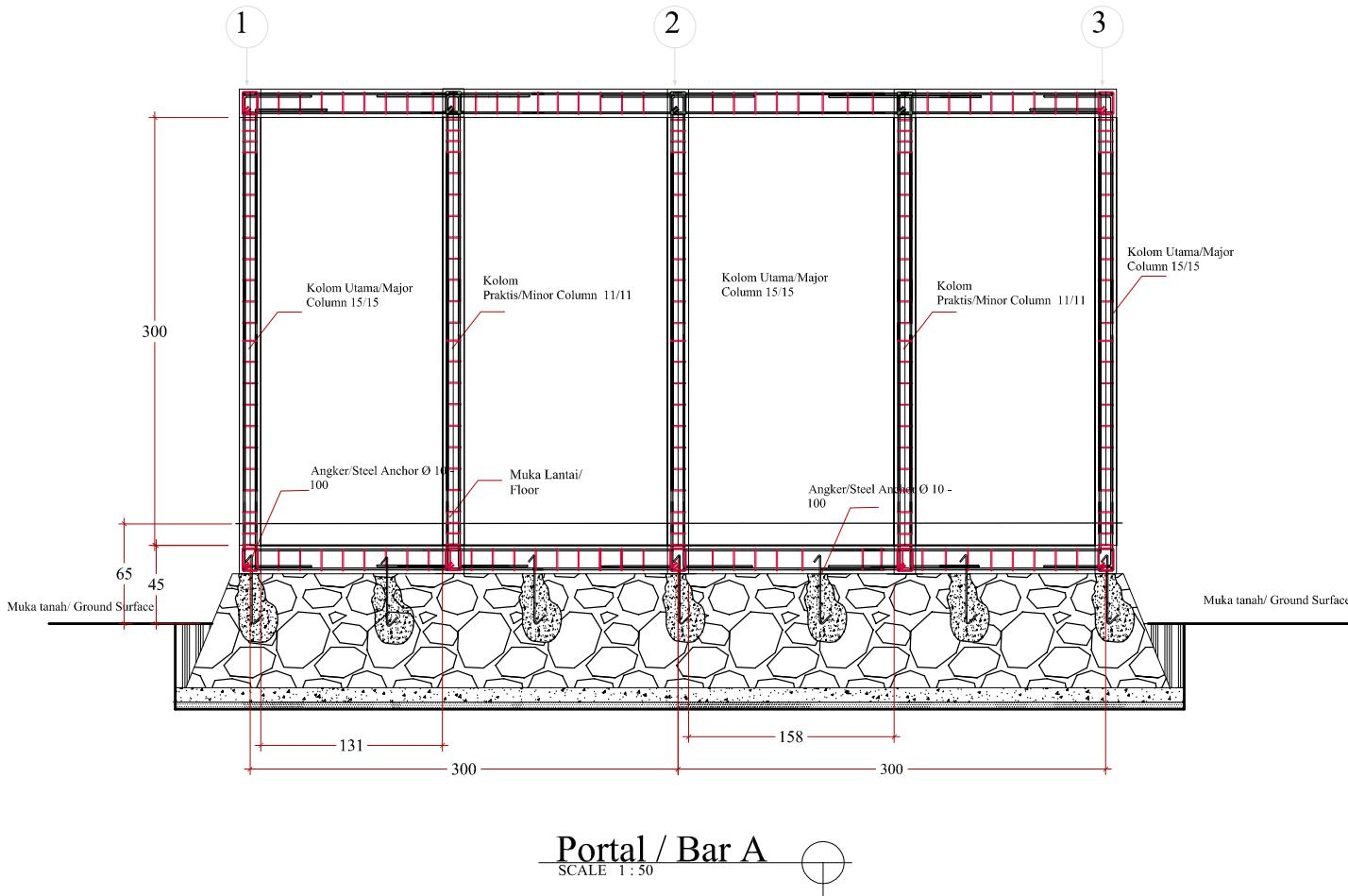
**NOTE** : This is a confined masonry house. masonry wall should be built prior to casting the column to ensure a good connection between wall and column.
