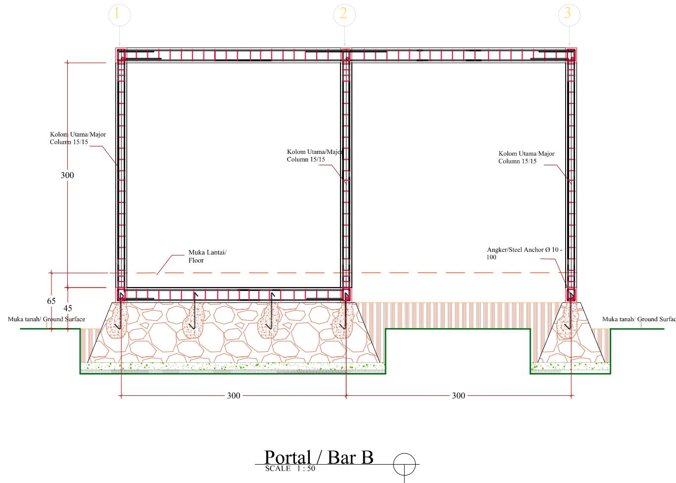
**NOTE** : This is a confined masonry house. masonry wall should be built prior to casting the column to ensure a good connection between wall and column.
