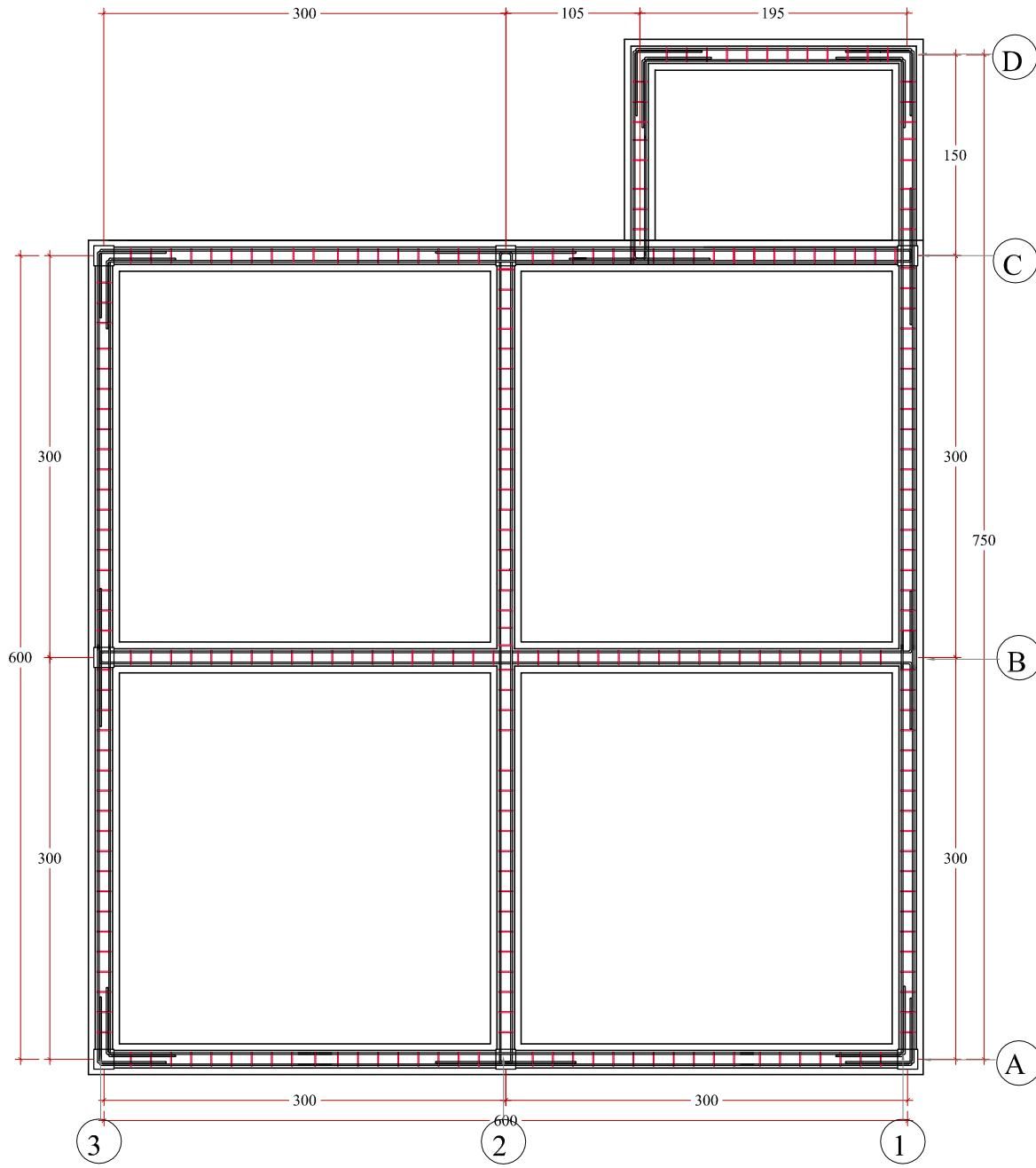
Denah Pembesian Ring Balk/Lay Out of Ring Beam Bar
