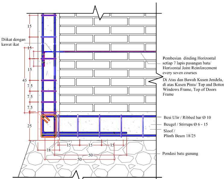
Rencana Pembesian Dinding/Beam to Column Joint
