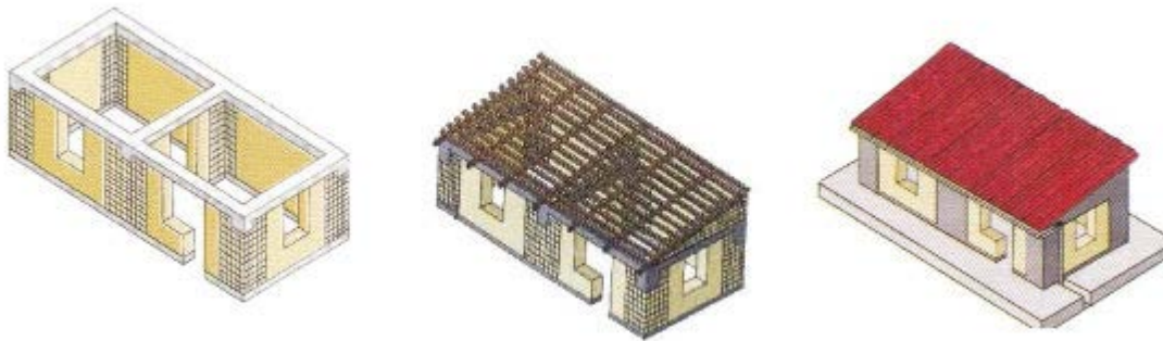
Fig 6. House design for reconstruction programme. Incorporates steel wire mesh at intersection of orthogonal walls, RC ring-beam and raft foundation (San Bartolome)
