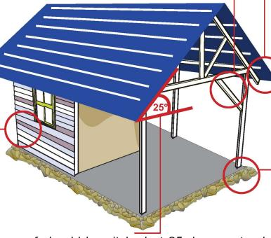
The roof should be pitched at 25 degrees to shed rain effectively. Rumbia is better than CGI sheets for a transitional shelter as it keeps the small space cool in the sun. To reduce heat transfer, cover sheets with rumbia or paint them white.
