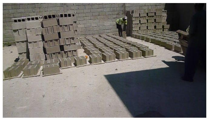
The common practice of leaving the blocks in the sun to dry severely affects the proper curing of the block and is reflected in a lower final compressive strength.
