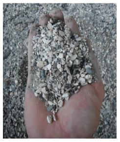
"Concassé" performs very well in block production. Rocks are hard and highly angular with low amounts of fine materials. Block makers can produce "Concassé" by carefully selecting rocks from the river or quarry and milling them onsite.
