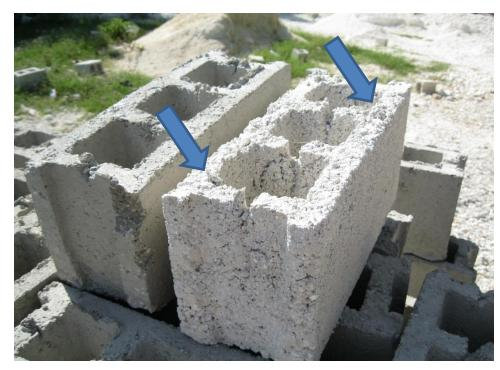
A rough finish on the top and sides of the block (RIGHT) is an indication of insufficient general compaction.
