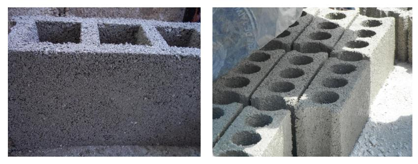
A smooth and regular finish on the top and sides shows good compaction throughout the block.
