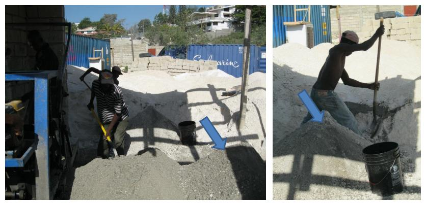
A block is only as strong as it's weakest part, so an even and regular mix is extremely important. This block maker does not mix well enough, leading to a substandard block (4MPa).
