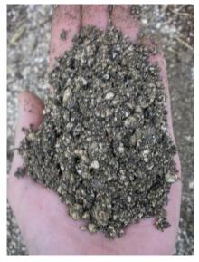
River sand must be washed and sieved to remove silts and organic debris. Particles are noticeably rounder from erosion.
