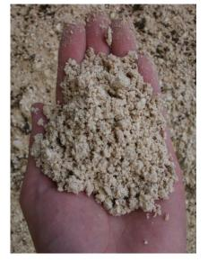
Quarry sand is mainly from two varieties of limestone. Larger particles are angular but can be soft and caked in dust. Washing is recommended. Despite a high percentage of finer particles good results can be achieved with this sand.
