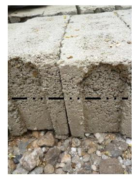
"Bands" of different smoothness indicate a mix of compacted and non compacted areas. A block is only as strong as it's weakest point!
