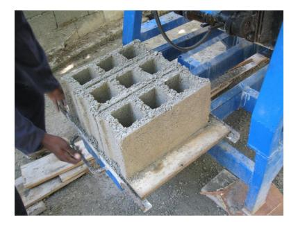
This reduces the material needed for each block and increases daily production. Though research is still being conducted on this practice, it is believed to have a large negative impact on the final compressive strength of the block.
